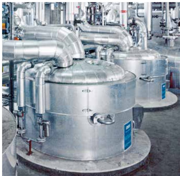
Niacin production plant, Visp, charcoal filtration of Niacin
